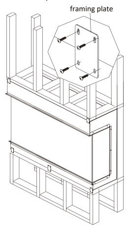
7. After checking that the fireplace operates properly, cover the glass panels with protective plastic bag and install plywood or drywall.
