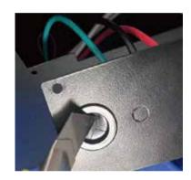
2. Attach the wiring to the junction block. Please make sure the live wire goes into the "L", the neutral wire into "N" and the ground wire into "G".
