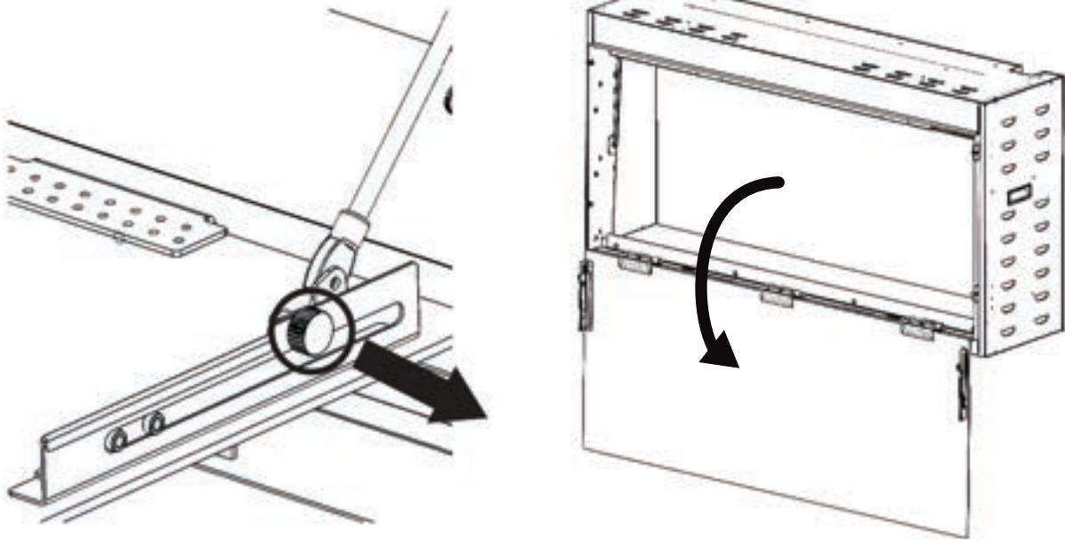
5. To remove the front glass, remove the screw holding the cylinder rod to the glass mount hardware. Note: The cylinders are no longer supporting the glass when screws are removed. Brace the glass while performing this action. Once the screws are removed, lift and close the glass in an upright position. Remove the screws holding the hinge to the glass bracket hardware. Once removed, the glass can be lifted from the firebox and placed on a soft, non-abrasive surface.
