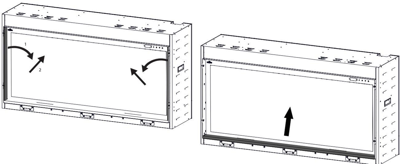
3. Remove the securing brackets at the top of the glass. Pull the glass outward using the provided suction cup. Alternatively, flip the securing brackets around to hook the top of the glass and pull outward.
