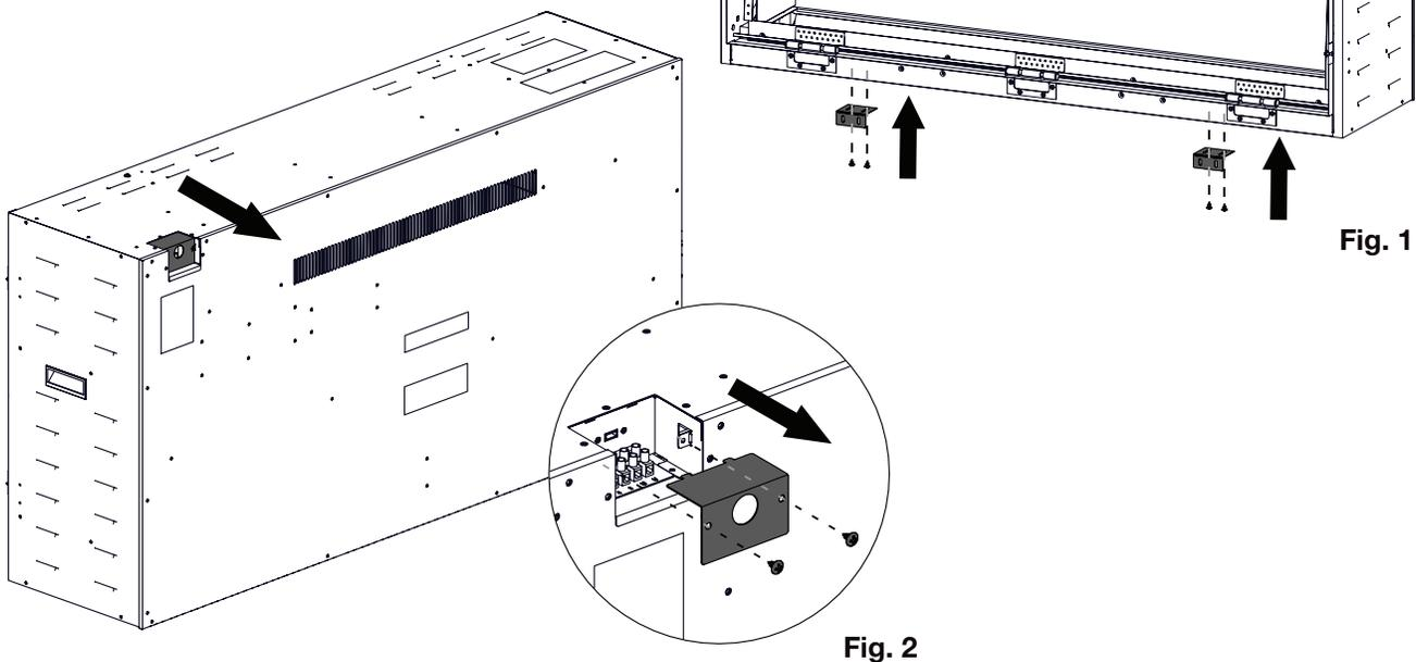
5. With the brackets installed, have 2 people lift the appliance up and insert the appliance into the rough in framing.
