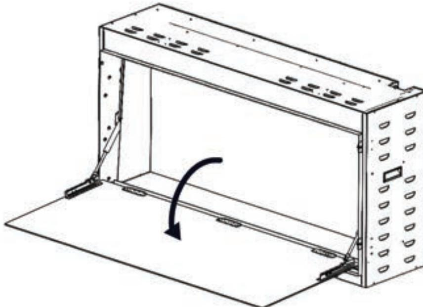
4. To fully open glass and fold down for easy service, remove the thumb screws on either side of the glass to allow the slides to engage. Note: The cylinders are no longer supporting the glass when the screws are removed. Brace the glass when performing this action and slowly allow the glass to swing down and come to rest.
