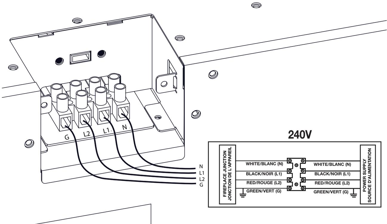
1. Insert Green or bare copper wire to the designated G Terminal. Tighten the screw.
