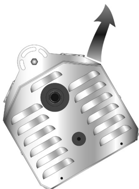
Figure 2.9 • Hot Flue Discharge
