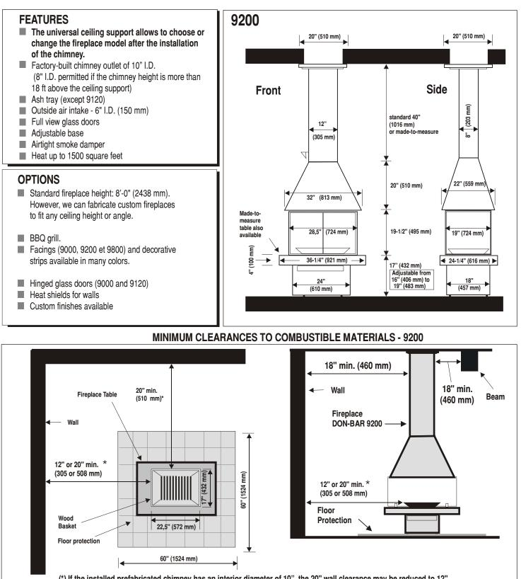
(\*) If the installed prefabricated chimney has an interior diameter of 10", the 20" wall clearance may be reduced to 12".
