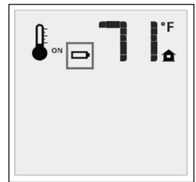
Figure 17: Low Battery Indicator.
