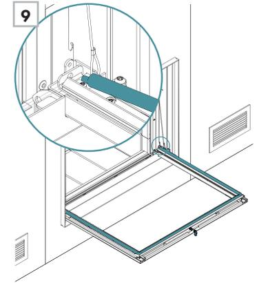
**Step 10** Slightly lift the door (45°) and slide up the glass 4" secure the frame by piercing the seal with the screw, do not tighten too much so the seal doesn't lift at all angles. Hand tighten is perfect.
