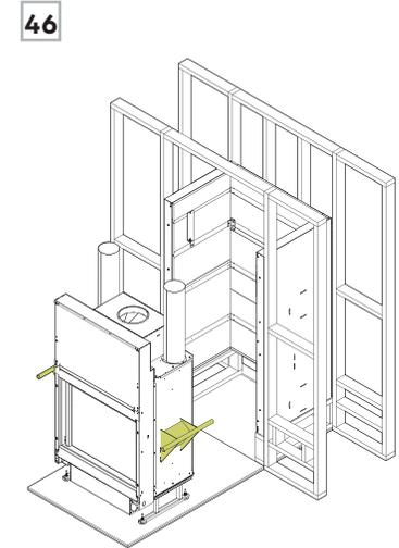
**Step 47** Move the fireplace into its final position inside the insulated shell.
