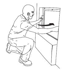
**Step 1** Take the firescreen by the wood handles and insert the vertical tabs as far as possible under the front portion of the fireplace.
