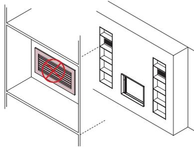
It is important that the airflow be continuous. It is forbidden to take fresh air from a closed room and to discharge the same airflow into another closed room.
