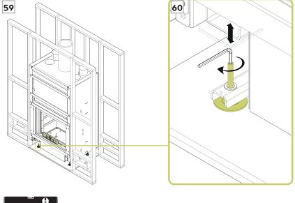
Step 61 Without the adjustable stands, legs cans be adjusted at the four corners inside the combustion chamber.
