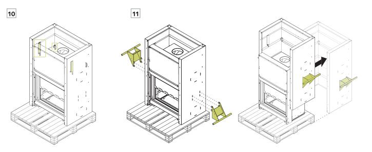
**Step 12** Locate and remove the 4 support brackets that hold the unit to the pallet.
