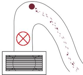
It is forbidden to have a curtain or any other object that can block the airflow located less than 24" in front of the hot air outlet, as air could get trapped behind it creating a heat trap.
