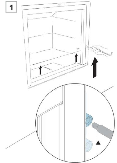
**Step 1** Using the fireplace handle provided with the unit, slide the glass up.
