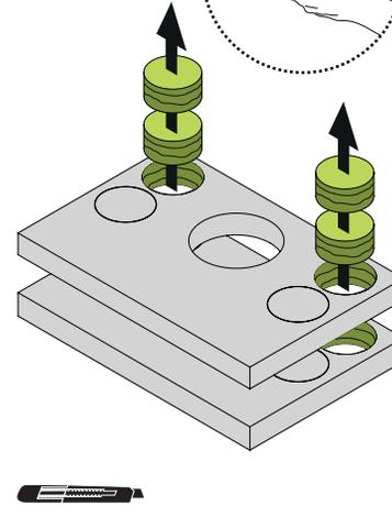
**Step 57** Replace the wool support plate and the two layers of wool around the convection flanges.
