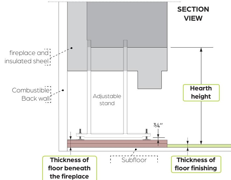
**Step 15** The minimum height requirement when installing an airtight box is  $10 \frac{3}{4}$ " from under the fireplace to floor. If the stands are cut too short the airtight box will touch the floor and will be damaged.
