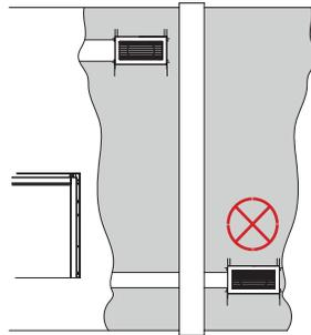
The hot air duct must always be installed horizontally or ascending as hot air naturally goes up, never down.
