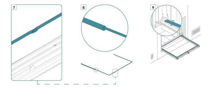
**Step 10** Slightly lift the door (45°) and slide up the glass 4" secure the frame by piercing the seal with the screw, do not tighten too much so the seal doesn't lift at all angles. Hand tighten is perfect.
