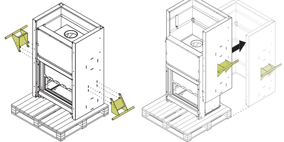
**Step 12** Locate and remove the 4 support brackets that hold the unit to the pallet.
