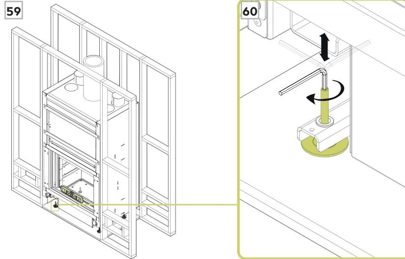
**Step 61** Without the adjustable stands, legs can be adjusted at the four corners inside the combustion chamber.
