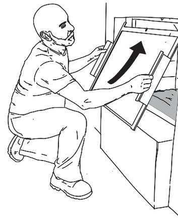
**Step 1** Take the firescreen by the wood handles and insert the vertical tabs as far as possible under the front portion of the fireplace.
