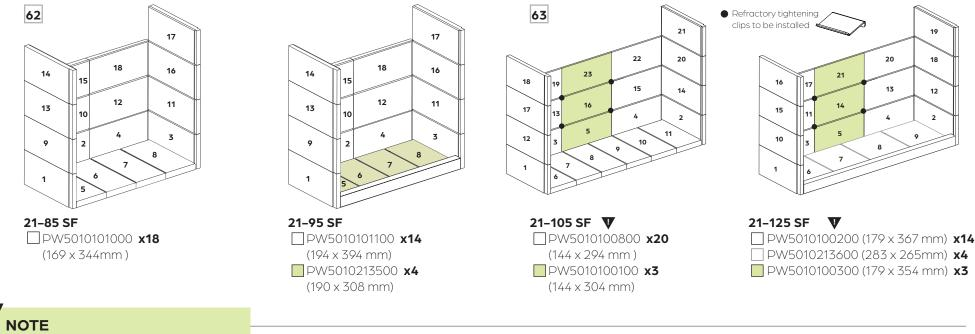
For 21-105 SF and 21-125 SF only, if the refractory bricks on the back seem unstable follow the steps on the next page for installation of the tightening refractory brackets.
