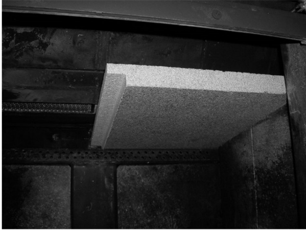
Figure 18 (cont.) - Removing/Replacing the Baffle for Inspection
