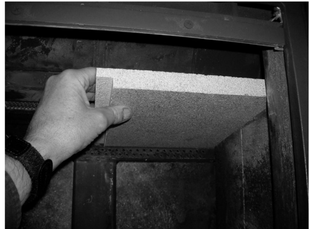
Figure 18 (cont.) - Removing/Replacing the Baffle for Inspection
