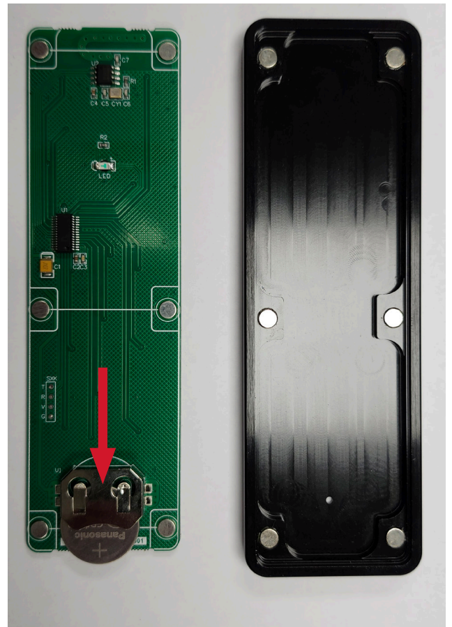
Figure 30: Remote Battery - Step 3
