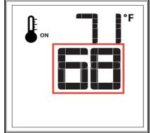
To activate this option, press the "Thermostat" key. To adjust the desired temperature, use the "Up" or "Down" until the desired temperature is displayed on the remote LCD screen.
