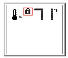
To activate this feature, press the "Mode" and "Up" at the same time. A lock icon will appear in the LCD screen. To deactivate this feature, press the "Mode" and "Up" at the same time.
