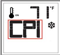
When the system is Off pressing the "Mode" key to index to CPI mode icon. Press the "Up" arrow will select the CPI mode (but it is still not activated. See instructions at link above)
