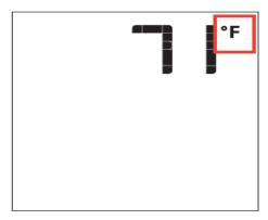
To change from in Fahrenheit (°F) to Celsius (°C.), or vice versa, press the **"Thermostat"** key and the **"Mode"** key at the same time.
