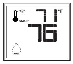
To activate the smart thermostat function, press the "Thermostat" key while the appliance is on until the word SMART appears beside the icon of the thermostat. To adjust the set temperature, press the "Up" or "Down" arrow keys until the desired temperature is displayed on the LCD.
