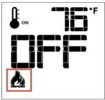
By pressing the "Down" key once it will reduce the flame height by one step. Continued pressing of the down arrow will result in the unit turning off. To return to normal fireplace operation use the "Up" key to increase the flame height to high. If the "Up" has been pressed while the system is ON, but the flame is OFF the flame will come ON in the high position.
