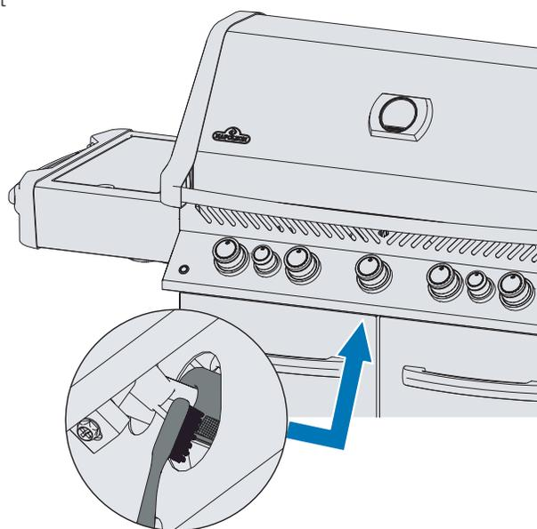
**WARNING!** It is very important the valve/orifice enters the burner tube when reinstalling the burner after cleaning and before lighting your grill, or a fire or explosion could occur.
