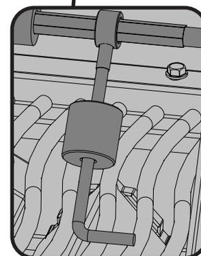
Ensure stop bushing is tightened on the inside of hood casting.
