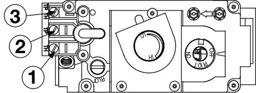
Disconnect the existing wires from terminals 1 and 3 (from the ON/OFF switch) and replace with the leads from the wall switch / millivolt thermostat.
