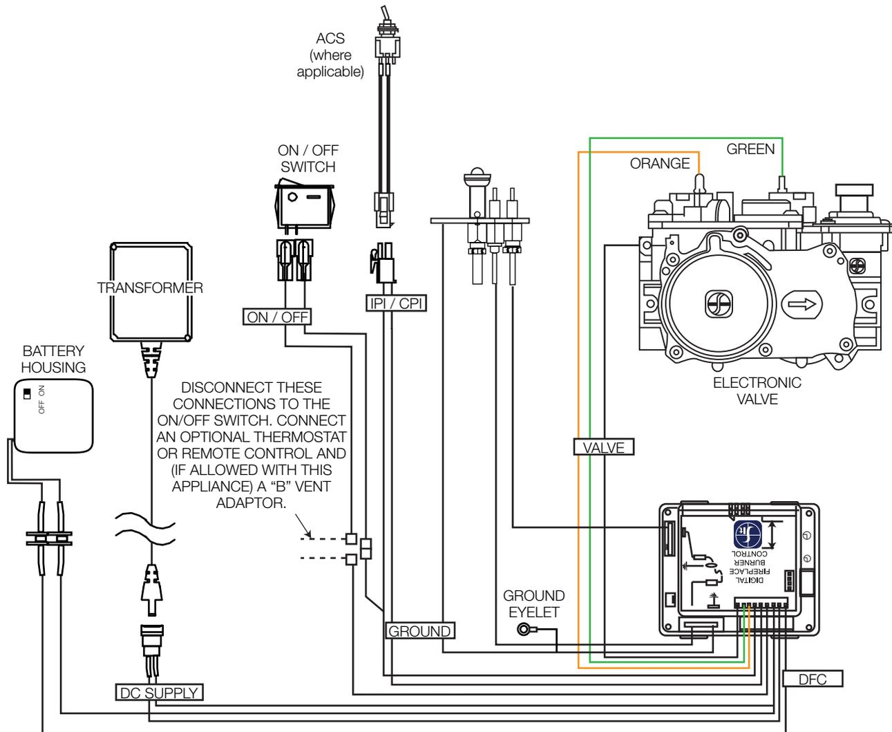
WHERE APPLICABLE, APPLIANCES WITH "B" VENT ADAPTORS MUST HAVE THE SPILL SWITCH WIRED IN SERIES WITH EITHER THE EXISTING SWITCH OR OPTIONAL WALL SWITCH, THERMOSTAT OR REMOTE.
