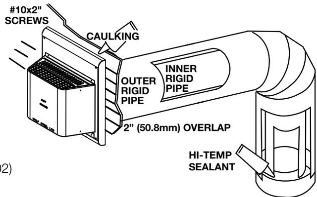
**The air terminal mounting plate may be recessed into the exterior wall or siding no greater than the depth of the return flange.**
