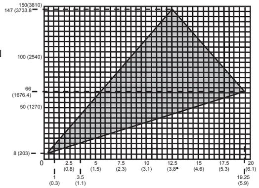
HORIZONTAL VENT RUN PLUS OFFSET IN FEET (METERS) H<sub>T</sub>
