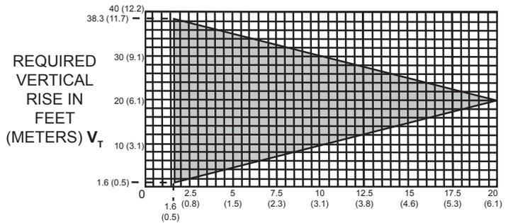
HORIZONTAL VENT RUN PLUS OFFSET IN FEET (METERS)  $H_T$
