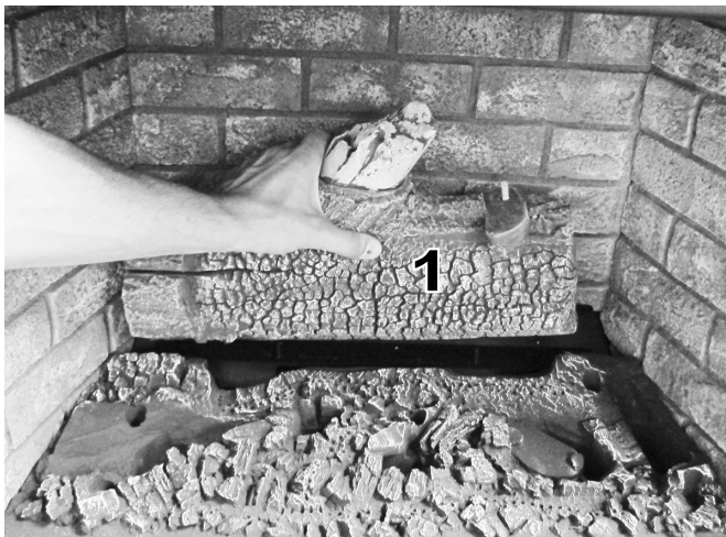
Figure 31. #1 Log. Engage the two pegs located on rear burner skirt with the holes in the underside of the log.
