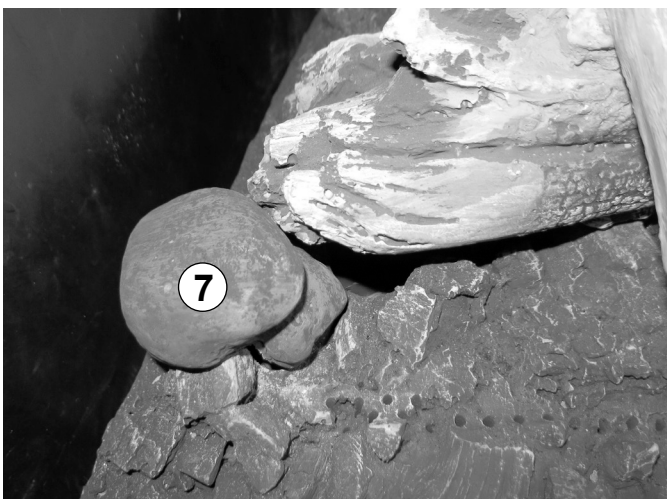
Figure 7.32. Engage blocks in the underside of Right Lower Rock #1 with the adjacent pockets on the burner base by Log #2.
