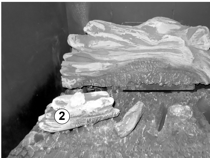
Figure 7.28. Engage the two pockets in the underside of Left Lower Log #2 with the two adjacent blocks on the burner base.
