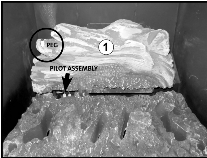
Figure 7.26. Engage the Rear Log with the two pegs located on rear burner skirt.
