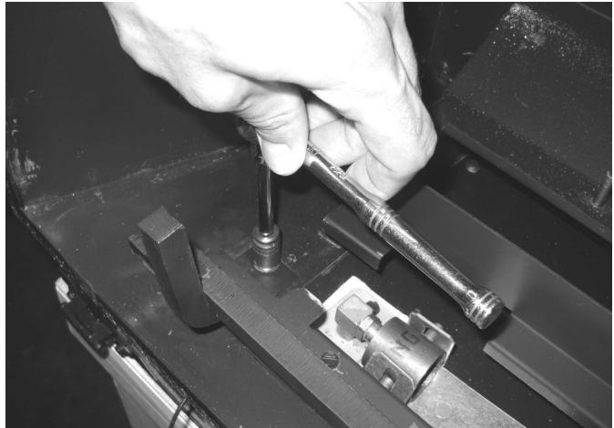
Figure 21. Remove left side Grate assembly M6 nut...
