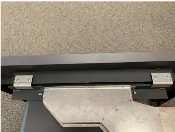
Surround hooks hanging the surround on the frame.
