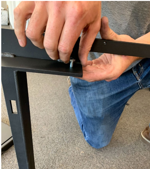
Preset set the 2 screws into the frame top for easy installation.
