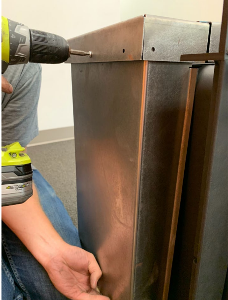
Attach the side blower duct piece to the top rear piece
