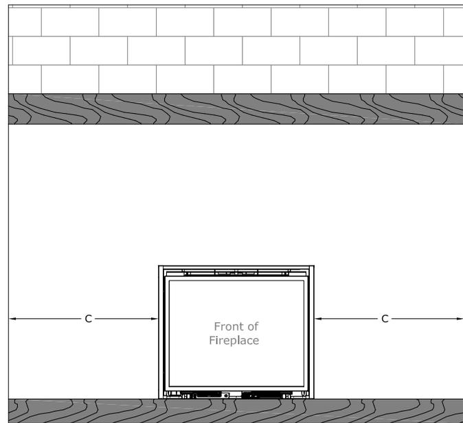
The width of the overhang to each side of the appliance (C) must be a minimum of  $\frac{1}{2}$  or greater of the roofline elevation (B) above the base of the fireplace.
