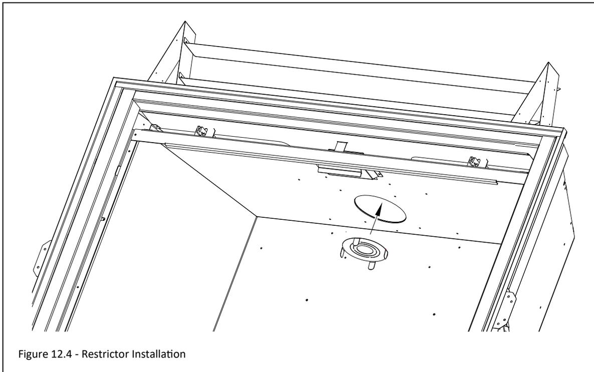
Figure 12.4 - Restrictor Installation
