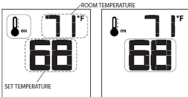
Figure 11.7 - Thermostat Operation
