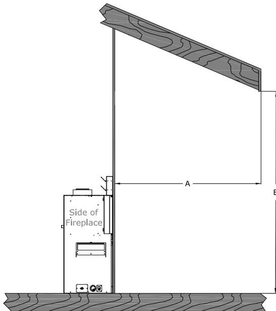
The overhang (A) must be a minimum of  $\frac{1}{2}$  or greater of the roofline elevation (B) above the base of the fireplace.
