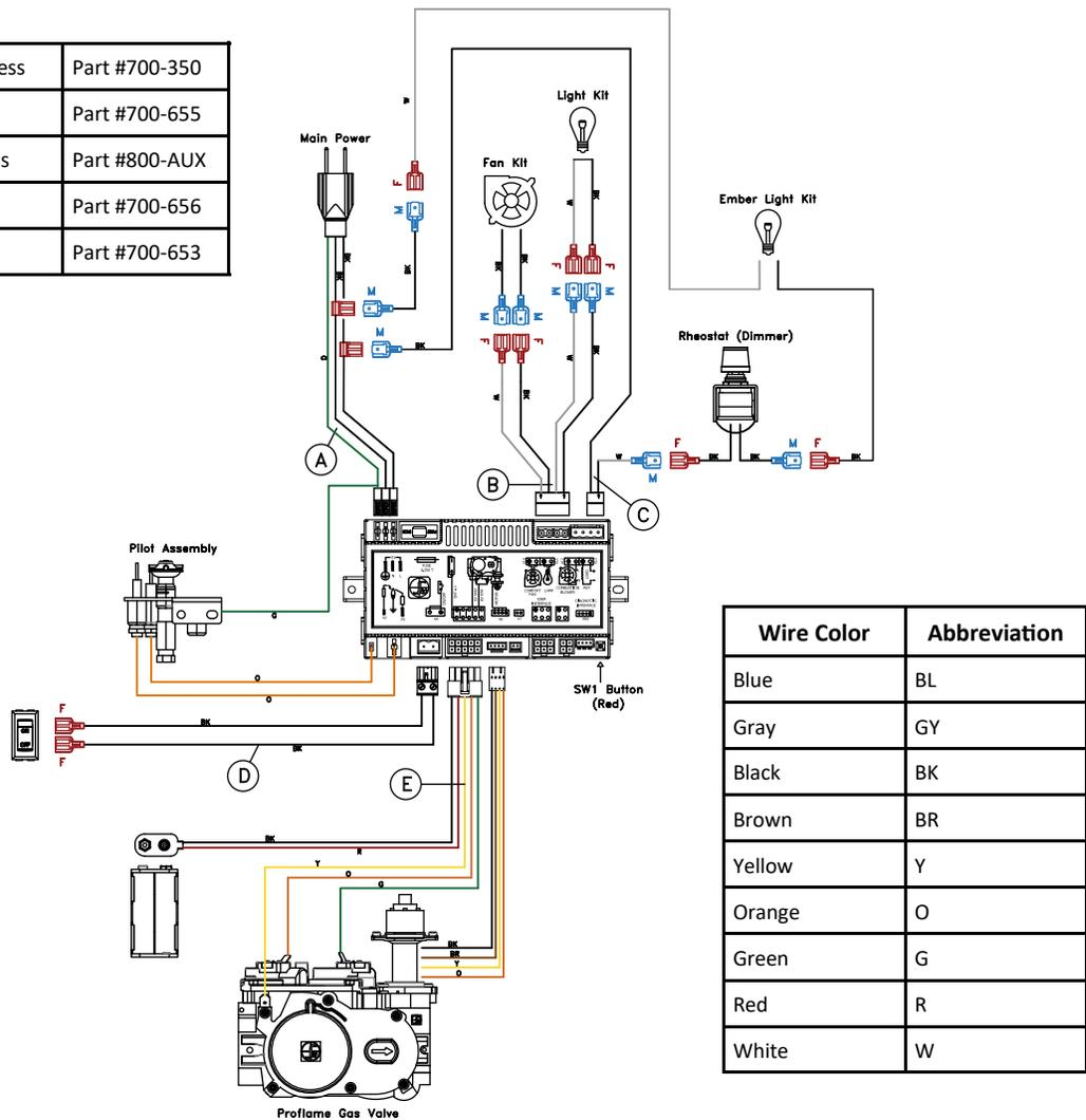
Figure 10.1 - Electrical Diagram
