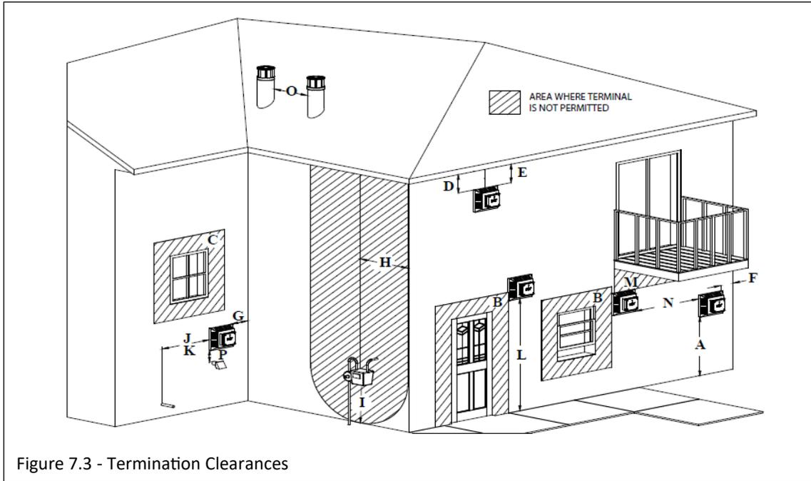
Figure 7.3 - Termination Clearances
