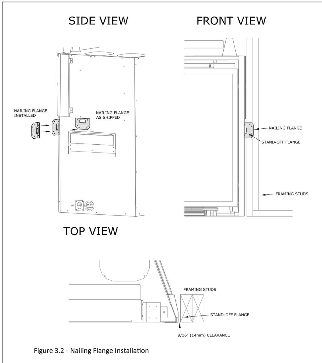
Figure 3.2 - Nailing Flange Installation
