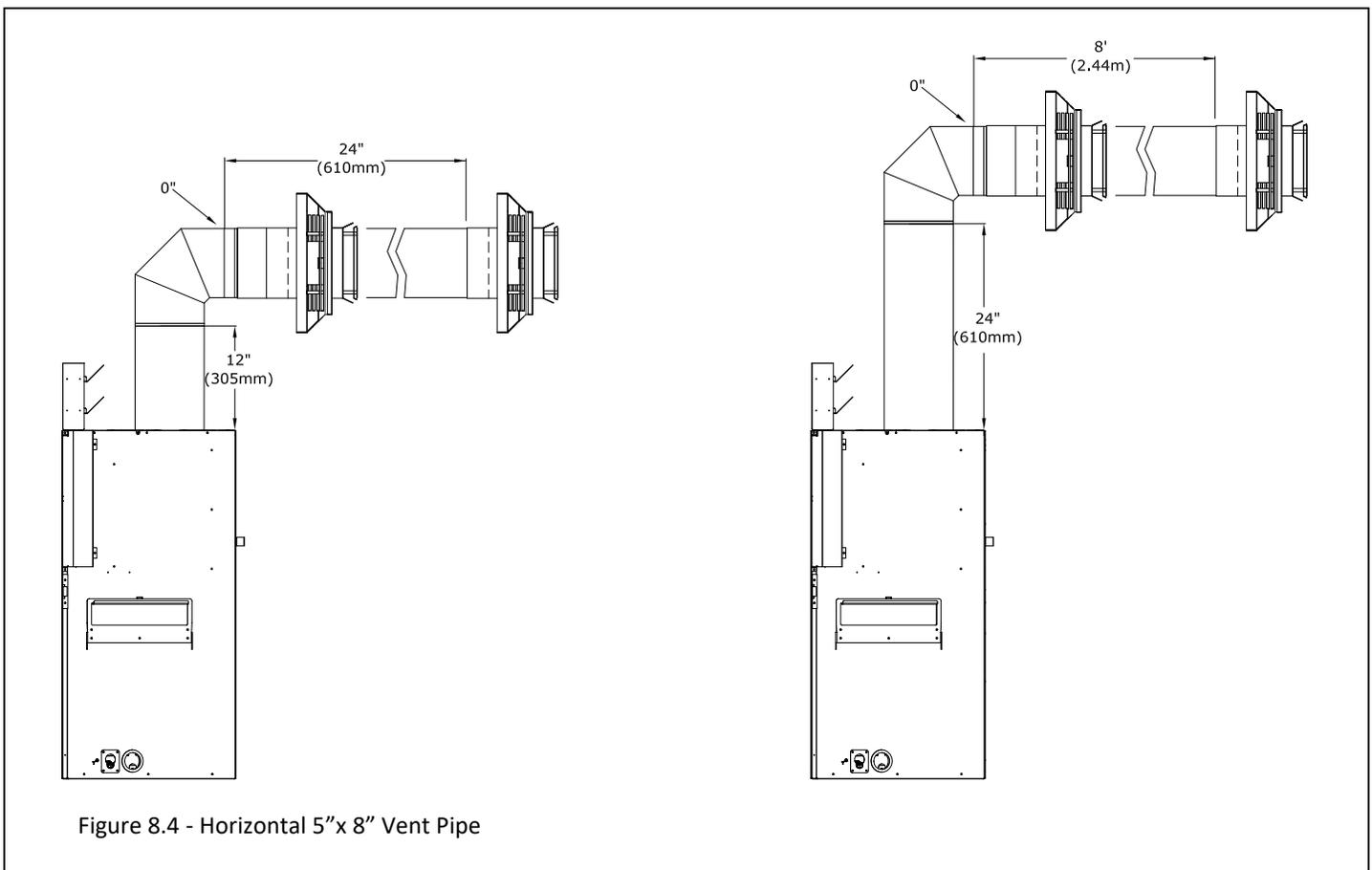
Figure 8.4 - Horizontal 5" x 8" Vent Pipe
