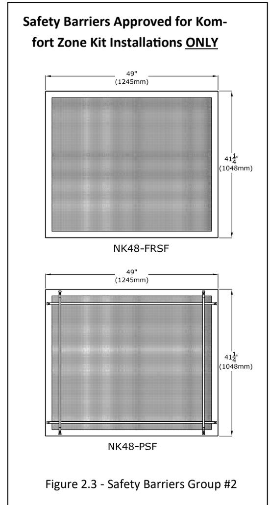
**IMPORTANT:** The NK48-PSF and NK48-FRSF (Figure 2.3) are ONLY approved for use when the Nordik 48 DV is installed with an approved Komfort Zone Kit (#KZK-045).
