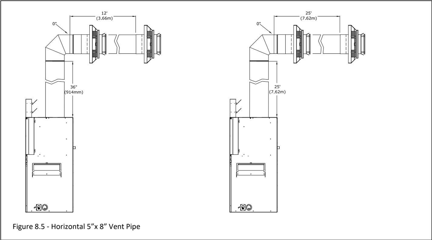
Figure 8.5 - Horizontal 5"x 8" Vent Pipe
