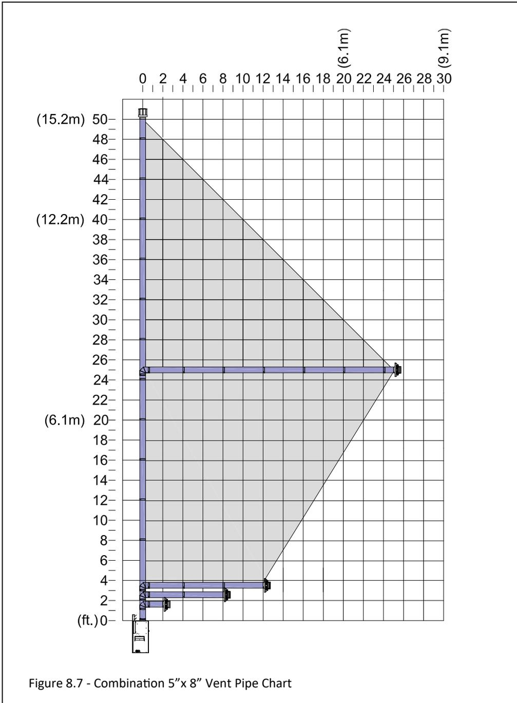
Figure 8.7 - Combination 5" x 8" Vent Pipe Chart
