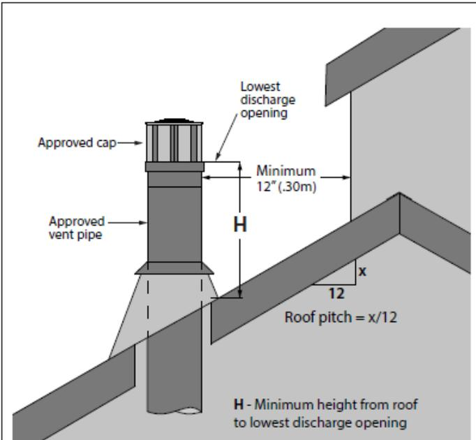
H - Minimum height from roof to lowest discharge opening
