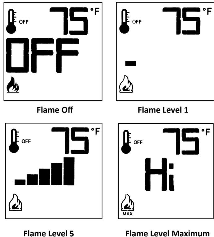
Figure 11.5 - Flame Adjustment
