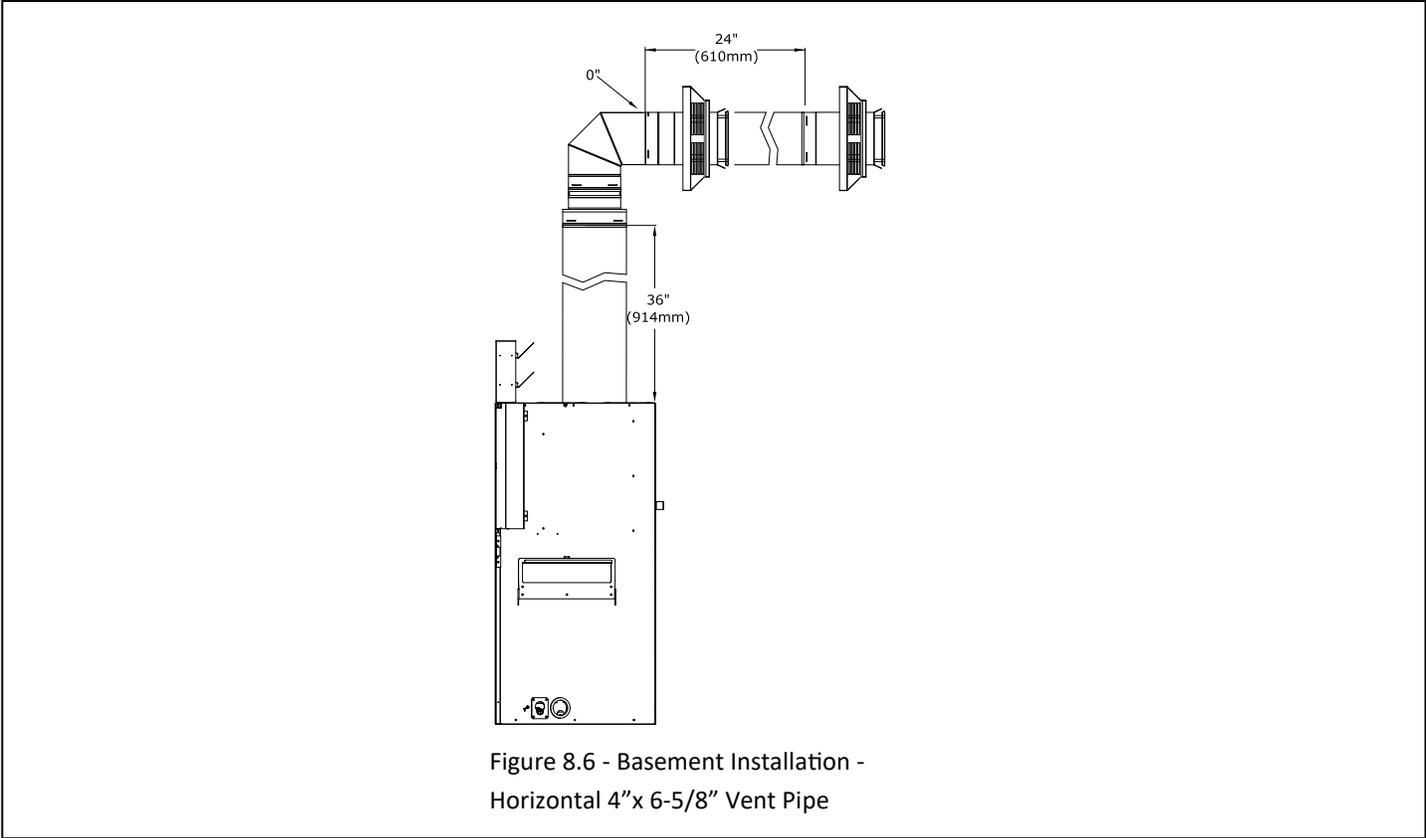
Figure 8.6 - Basement Installation - Horizontal 4"x 6-5/8" Vent Pipe
