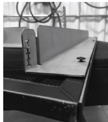
Figure 5.9 - Screen Barrier Louver Adjustment
