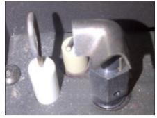
**Figure 15: Correct Pilot Position**
