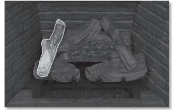
Figure 38: Log Set Installation - Step 5
