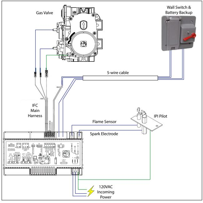
Figure 30: Wiring Diagram
