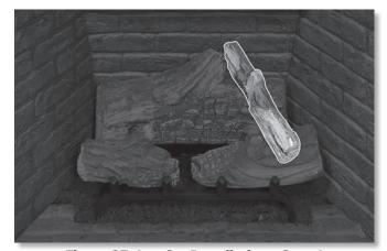
Figure 37: Log Set Installation - Step 4
