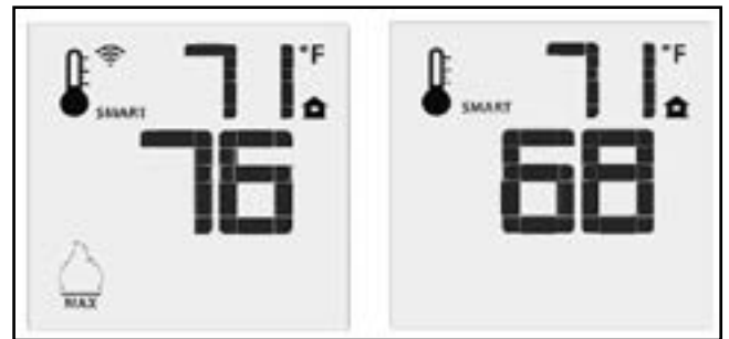
Figure 10: Remote Control's Smart Flame Function.
