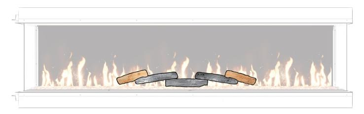
4. Select the 12" slim logs and stack these on the ends of the 12" big logs.
