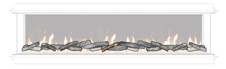
12. Use the bag of wood chips and place a few chips and chunks in the gaps between the logs. We recommend using these sparingly for the best appearance and to maximize the light output from the ember bed.
