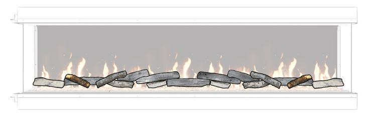
10. Select the last two 10" logs, and stack these laying over the 12" big logs. The inside end of the log may be the he flame screen and the outside end may be towards you.
