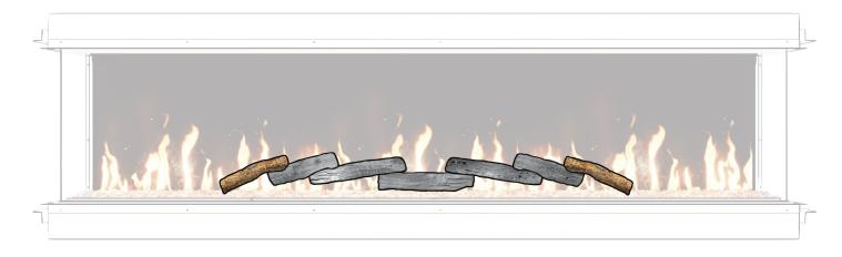
5. Select the last two of the 16" Accent logs, and rest them on the left and right of the 12" slim logs. The 16" filler logs should be resting on the ember bed.
