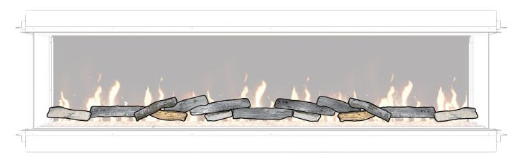
9. Select the 10" logs, and stack these laying over the 16" filler logs. The inside end of the log may be towards you and the outside end may be towards the flame screen.
