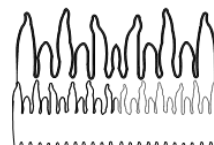
Dark, orange flames with black tips (Venturi closed too far. Open venturi slightly)
