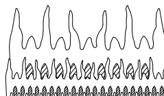
Lazy, yellow flames-no adjustment necessary (Ideal Flame Appearance)
