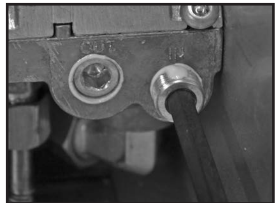
Figure 45: Testing port caps with thread sealant.
