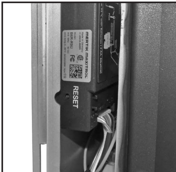
Figure 99: Maxitrol reset button location.
