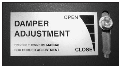
Figure 47: Damper adjustment indicator.
