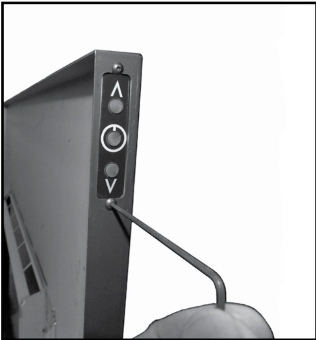
Figure 111: Attaching switch to backing plate.
