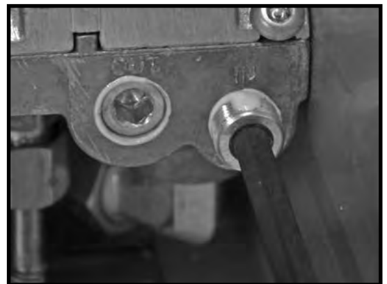
Figure 45: Testing port caps with thread sealant.
