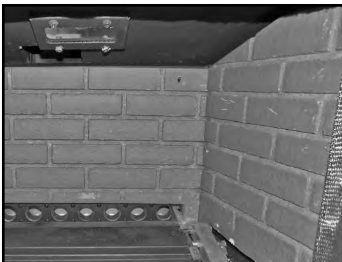
Figure 28: Right side panel in place.
