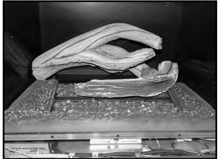
Figure 99: 2nd log placement.
