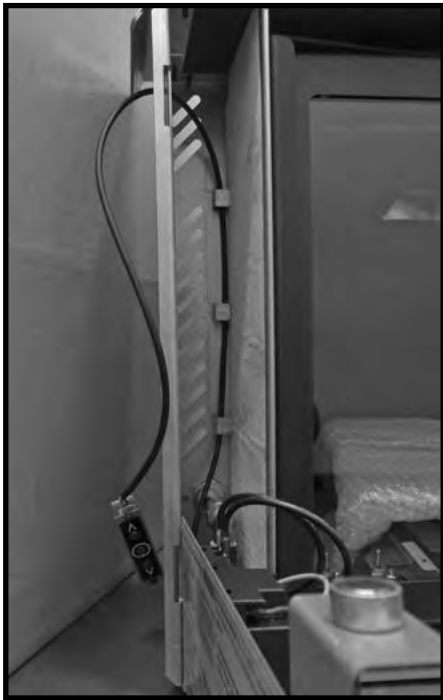
Figure 108: Pre-installed ON OFF switch assembly.
