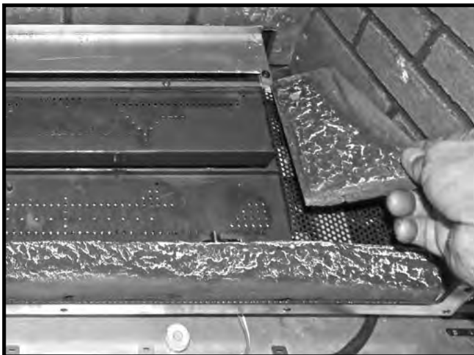
Figure 73: Right side base piece.
