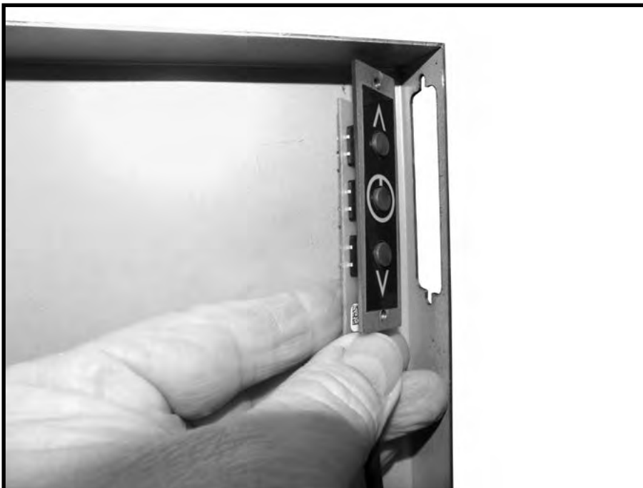
Figure 110: Positioning the switch behind the backing plate opening slot.
