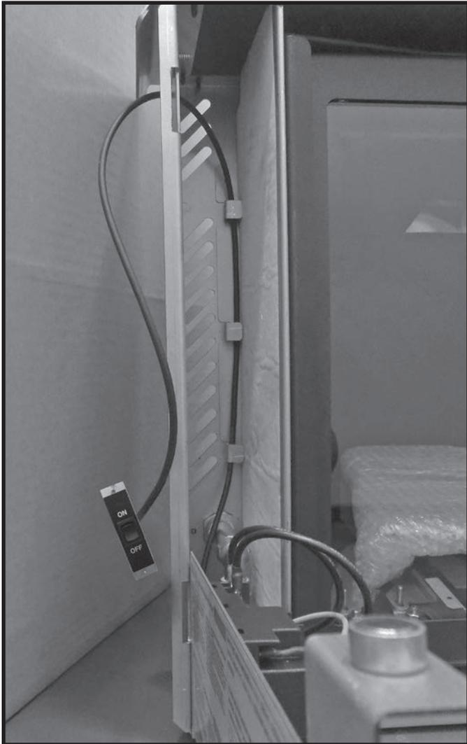
Figure 89: Pre-installed ON OFF switch SIT assembly.
