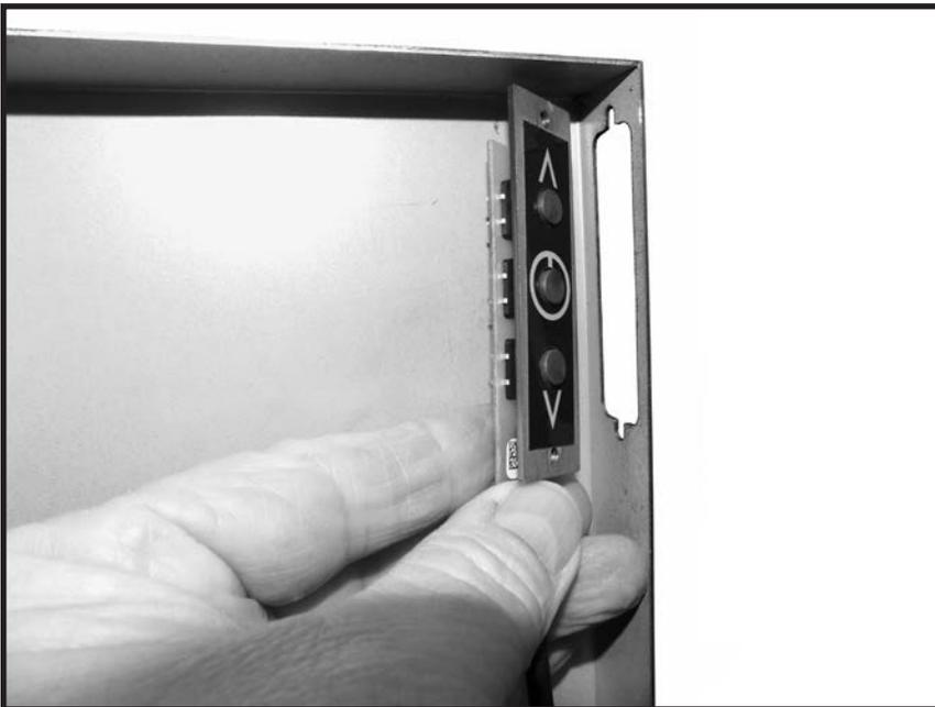
Figure 93: Positioning the switch behind the backing plate opening slot.
