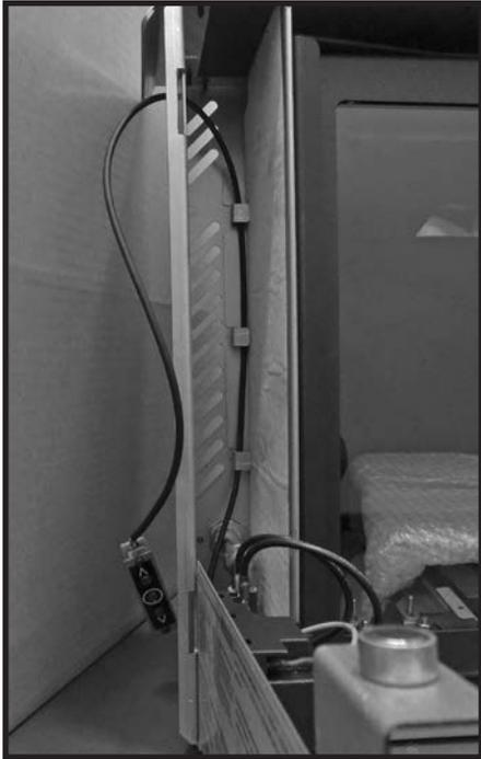
Figure 91: Pre-installed ON OFF switch assembly.
