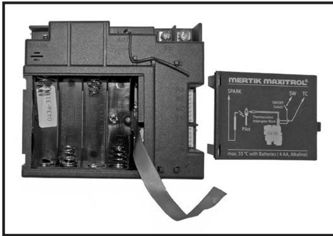
Figure 99: Maxitrol receiver module.
