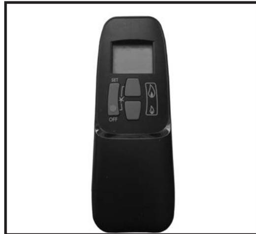
Figure 100: G6R remote control device.
