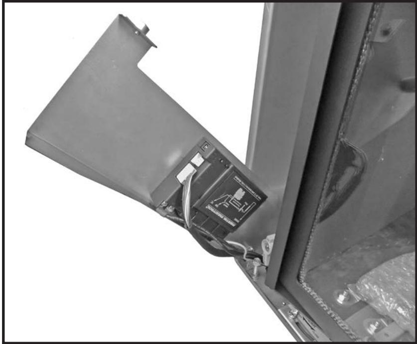
Figure 39: Maxitrol electrical controller in its caddy.
