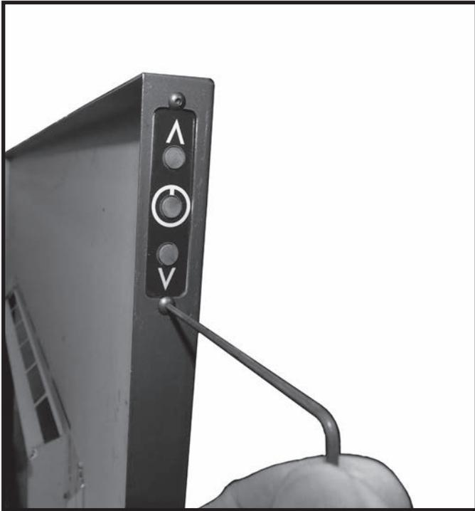
Figure 94: Attaching switch to backing plate.
