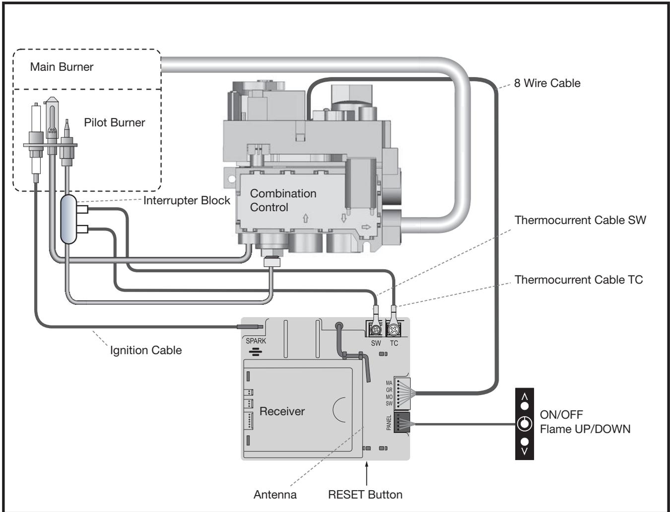
Figure 110: Maxitrol wiring diagram.
