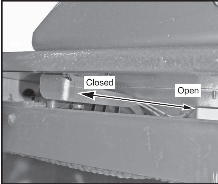
Figure 45: Damper adjustment.
