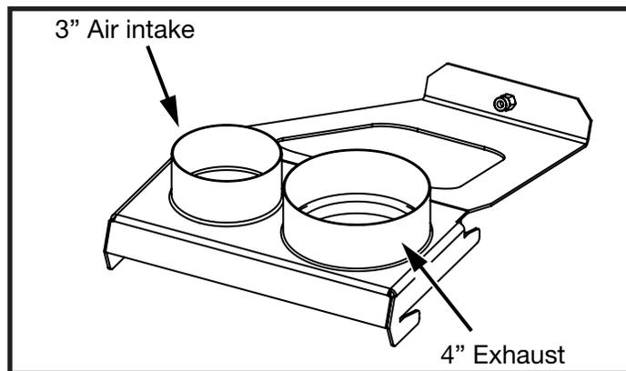
Figure 10: 4 x 3 inch Flue adapter.
