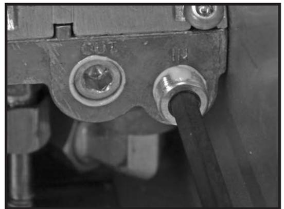
Figure 44: Testing port caps with thread sealant.
