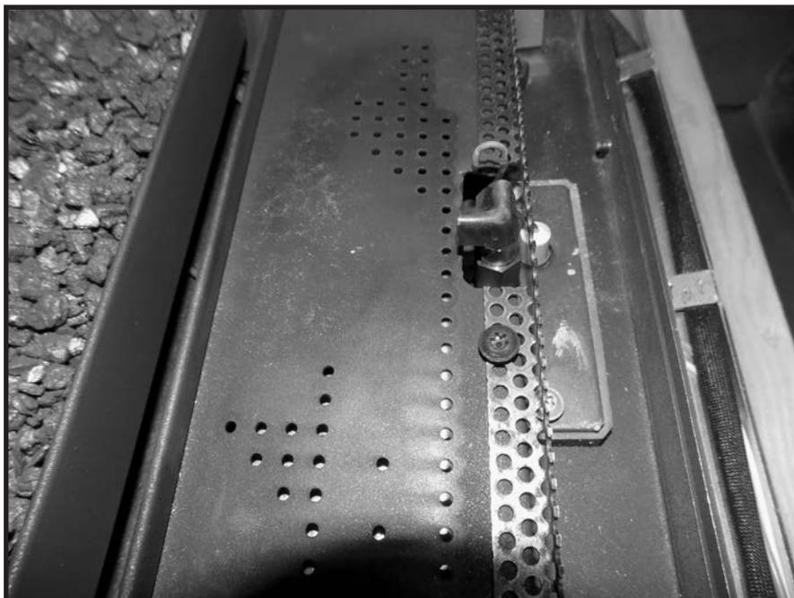
Figure 70: Front mesh guard in place.
