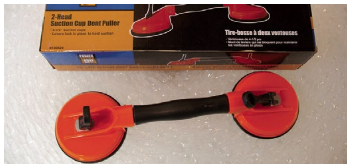
Figure 11.b Glass lifting tool
