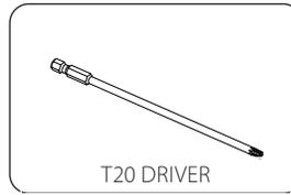
**17.** Install framing pockets to the the unit, using T20 fasteners. Ensure that the screen catches on the inside of the vertical pockets are situated towards the top of the unit.
