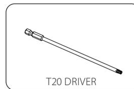
**7.** On the side and rear liner, remove the T20 fasteners securing liners to the firebox. Once the fasteners are removed you will be able to lift out the liners.
