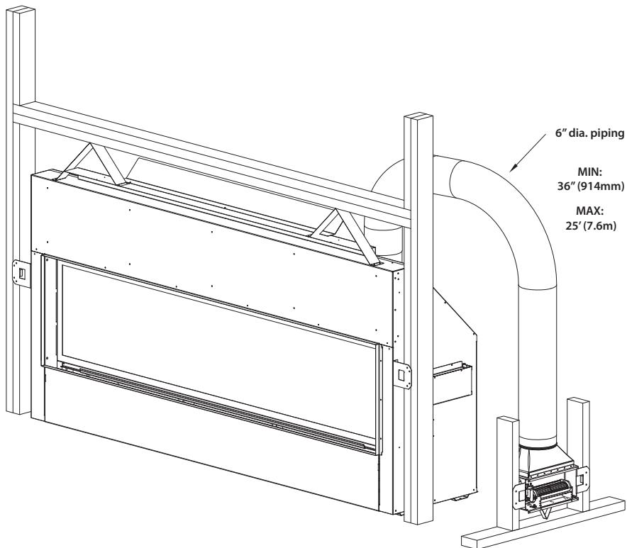
Figure 1.8, Piping Dimensions
