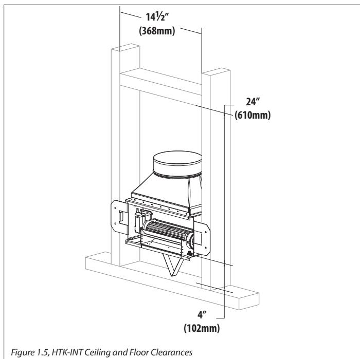
Figure 1.5, HTK-INT Ceiling and Floor Clearances
