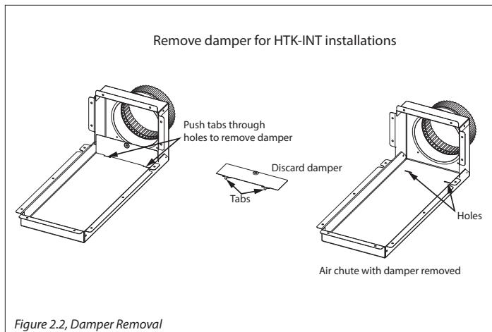
Figure 2.2, Damper Removal
