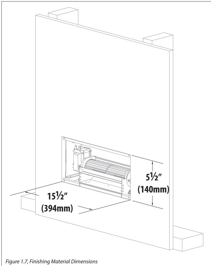
Figure 1.7, Finishing Material Dimensions
