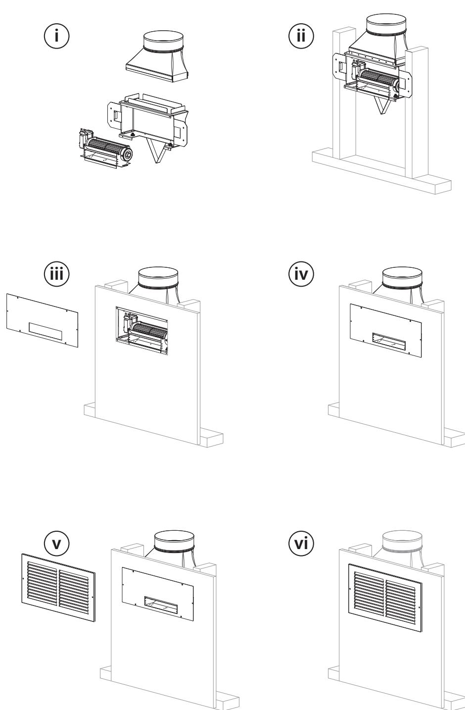
Figure 2.5, Fan Assembly Installation
