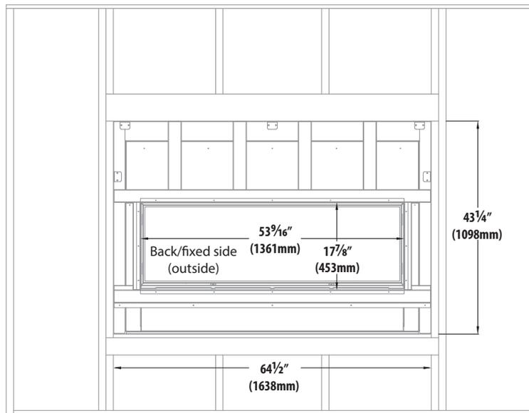
Figure 2.1, Framing Dimensions
