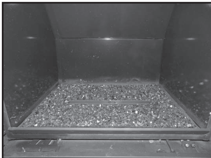
Figure 90: Crushed glass media in burner tray.
