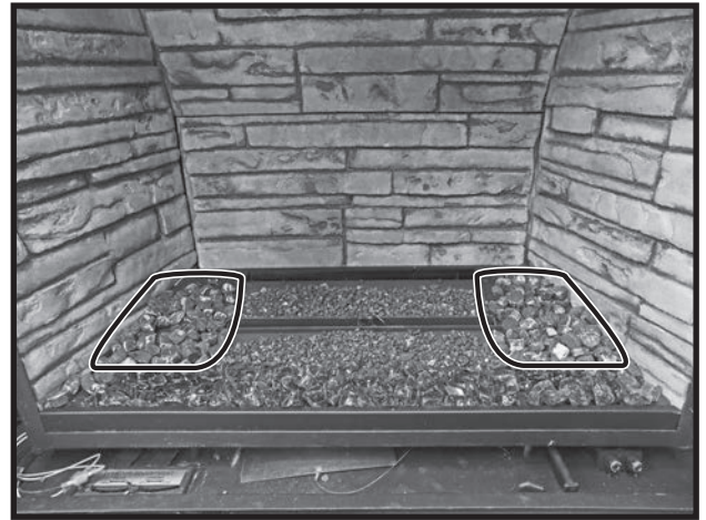
Figure 76: Large ember chunks on both sides of the burners.
