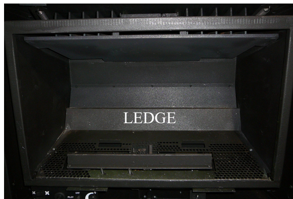
Figure 64: Back Brick Panel Ledge.
