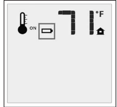
Figure 17: Low Battery Indicator.
