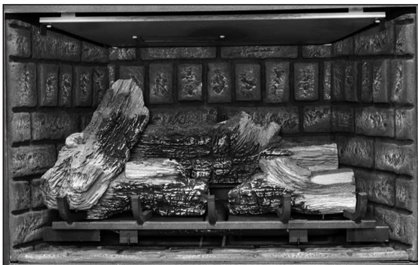
Figure 55: Place the left top log on the right, on top of the rear log and left mid log. Locate the bottom on the far left grate arm.
