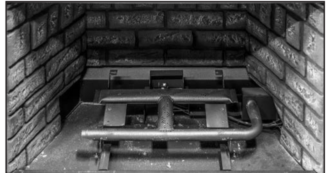
Figure 51: Remove the 6 screws highlighted in figure 50 using a Torx T-20 screwdriver and remove the air deflector
