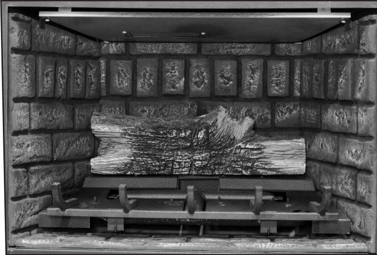
Figure 54: Install the back log on top of the pilot on the back shelf of the air deflector. Push it against the back brick panel.
