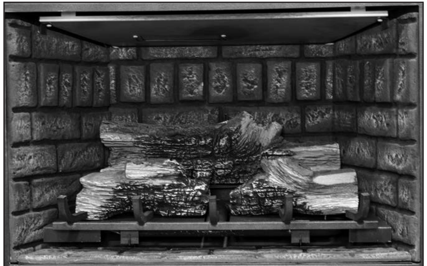
Figure 55: Place both the left and right mid logs in the middle of the air deflector. Make sure the bottom holes align with the pins in the air deflector.
