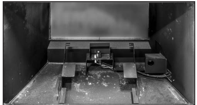
Figure 53: The rear liner can now be removed. Use a vacuum to clean up the bare firebox if needed.
