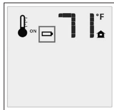
Figure 17: Low Battery Indicator.
