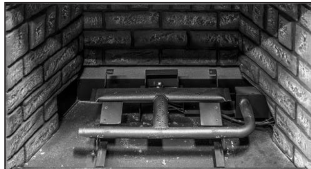
Figure 47: Remove the 6 screws highlighted in figure 46 using a Torx T-20 screwdriver and remove the air deflector
