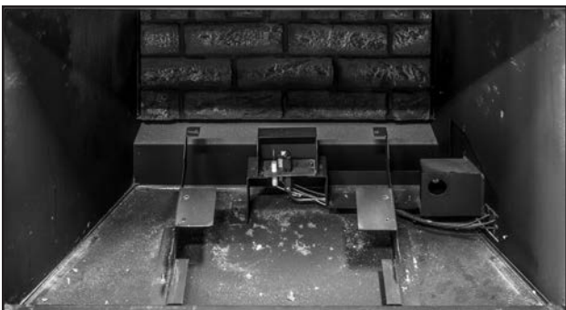
Figure 48: Lift the burner off the mounts and pull it out of the inlet box. The unscrew the panel brackets (T20's) from each side of the baffle to remove the left and right side liners.
