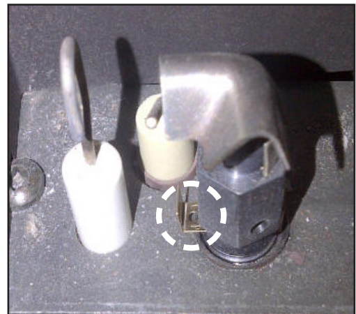
Figure 22. Pilot Slider set to LP
