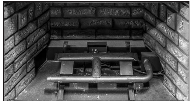
Figure 54: Remove the 6 screws highlighted in figure 53 using a Torx T-20 screwdriver and remove the air deflector
