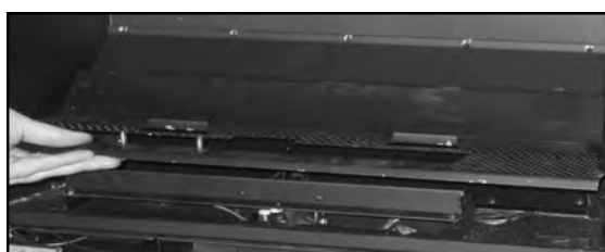
Figure 56: Burner Tray Installation.
