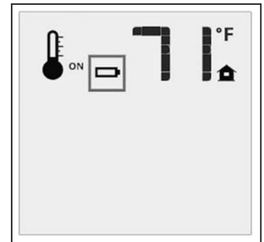
Figure 19: Low Battery Indicator.
