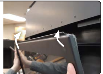
Figure 21.e Lift the door
