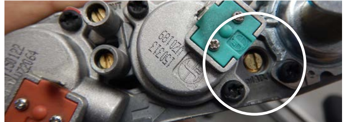
Figure 13.g Adjust pilot size
