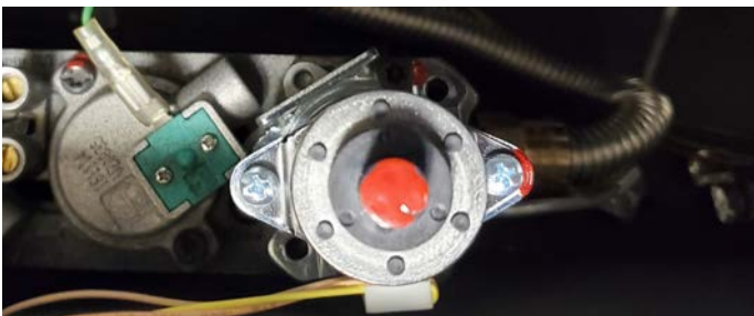
Figure 13.eee LP pressure regulator on a Full Load
