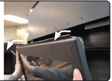
Figure 21.e Lift the door
