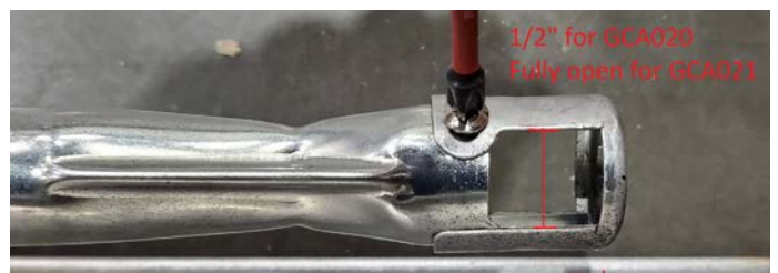
Figure 13.c primary air adjuster
