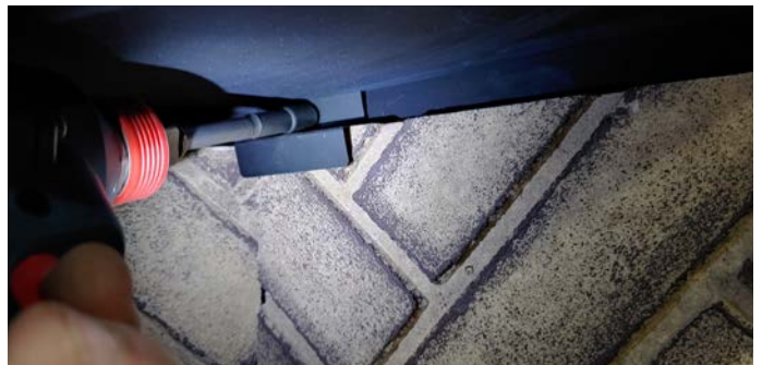
Figure 20.b Secure with the bracket using screw
