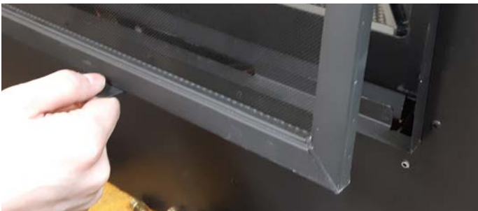
Figure 20.b Lift out the Retaining Tabs and screen
