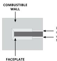
Leave ¼" gap between heat distribution kit opening and the wall. Gap will be covered with the faceplate
