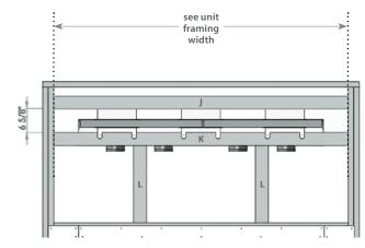
The opening should be a minimum of 38" from the top of the fireplace and a minimum of 3" from the ceiling. Secure with 12 wood screws (not provided)
