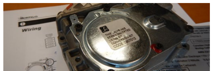
Figure 13.k Conversion label on valve
