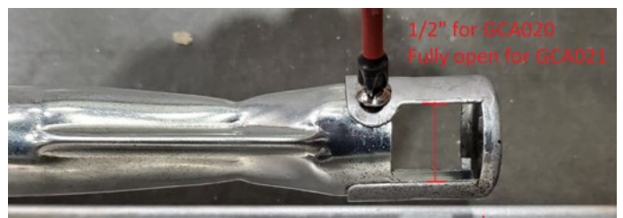
Figure 13.c primary air adjuster
