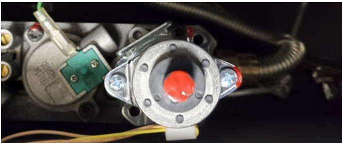
Figure 13.eee LP pressure regulator on a Full Load
