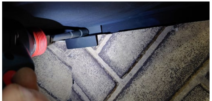
Figure 20.b Secure with the bracket using screw
