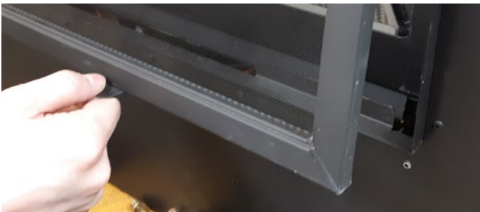
Figure 20.b Lift out the Retaining Tabs and screen
