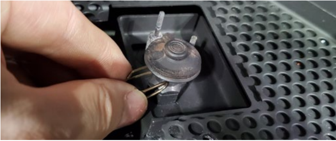
Figure 13.d Removing the spring clip
