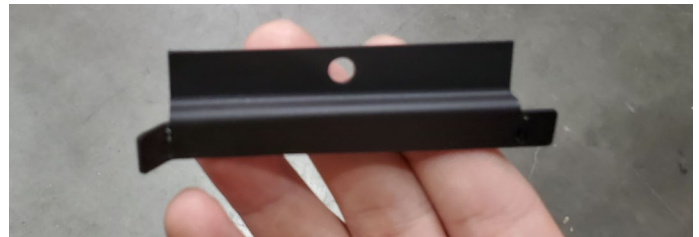
Figure 20.b Bend the left side tab
