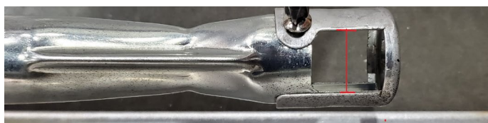
Figure 13.c primary air adjuster
