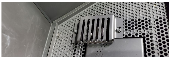
Figure 13. Removal of pilot cover
