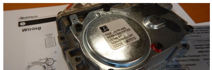
Figure 13.k Conversion label on valve
