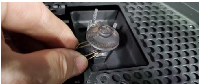
Figure 13.d Removing the spring clip
