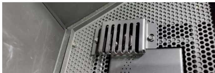
Figure 13. Removal of pilot cover
