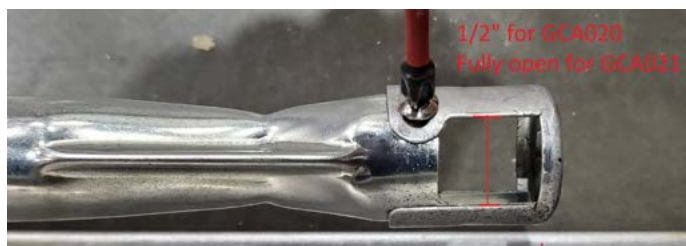
Figure 13.c primary air adjuster
