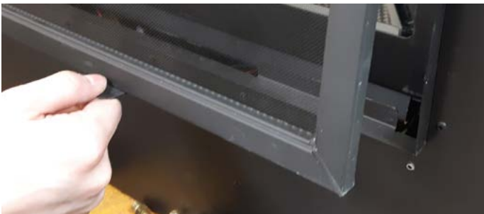
Figure 20.b Lift out the Retaining Tabs and screen
