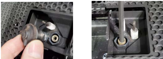
Figure 13.e Removing the pilot hood, orifice
