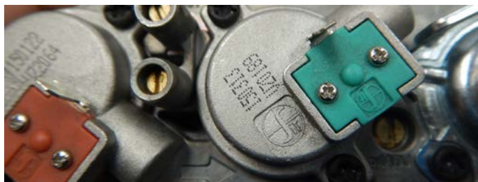
Figure 13.h Adjust pressure ports
