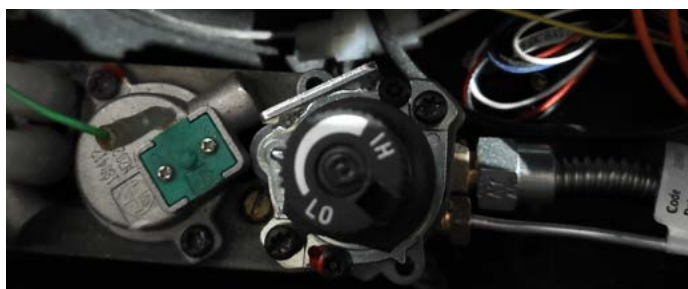
Figure 13.ee LP pressure regulator on Basic
