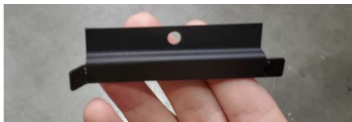
Figure 20.b Bend the left side tab
