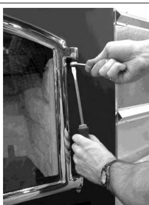
Figure 4 Door Hinge Adjustment
