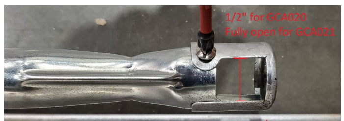
Figure 13.c primary air adjuster
