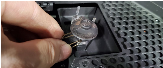
Figure 13.d Removing the spring clip
