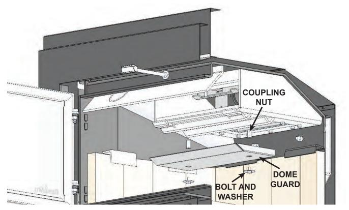
6. Remove the twelve remaining 1/4-20 nuts from the dome bottom. Lift the bypass door gasket retainer assembly upwards (enough to clear the threaded posts from the dome) and remove through the combustor opening. Once removed, ensure all debris is cleared from the inner surface of the dome.
