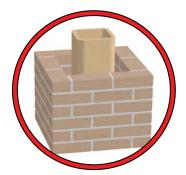
This appliance must be connected to a listed high temperature **(UL1777,ULC635,ULC640)** approved masonry chimney with a flue liner.
