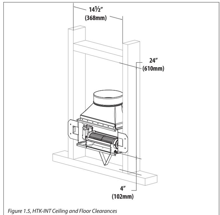
Figure 1.5, HTK-INT Ceiling and Floor Clearances
