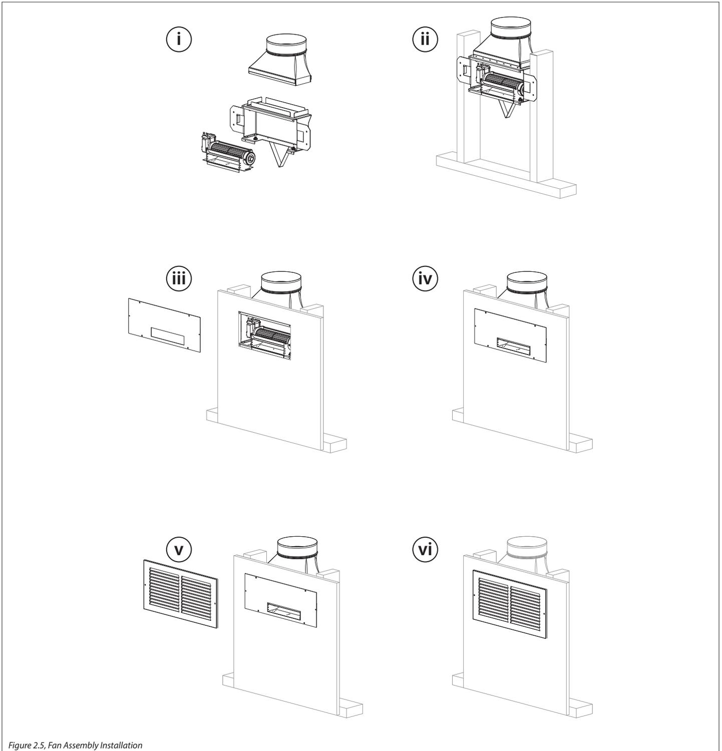
Figure 2.5, Fan Assembly Installation
