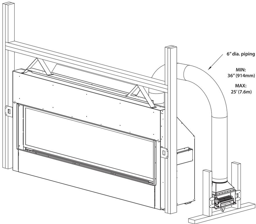
Figure 1.8, Piping Dimensions
