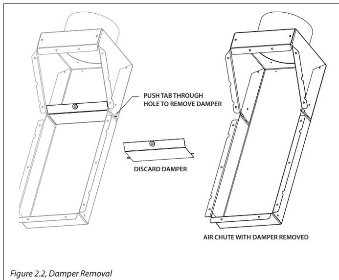
Figure 2.2, Damper Removal
